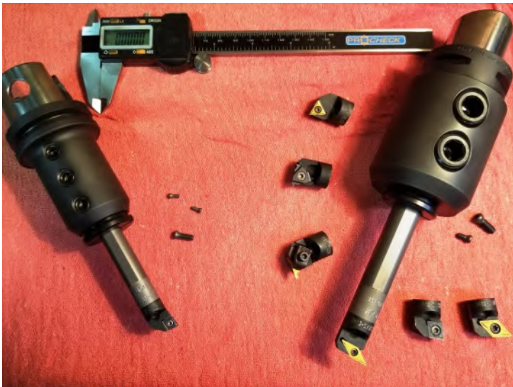
Versabar® Shanks Adapt To Capto® And KM Using A Boring Bar Adapter Combined With Split Sleeve Bushing
